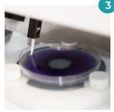
As the agar plate spins, the syringe automatically dispenses accurate volumes of sample.
