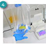
Pull the arm backwards. Open the holder, and take out the sample's plastic bag.
