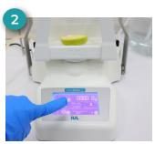
**Tare weight** and introduce the sample in the plastic bag.
