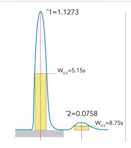
The graphic shows the absorbance peak for a 1-mg/kg mercury solution and the subsequent profile of blank run.
