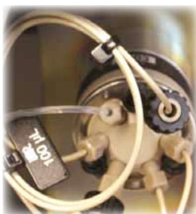
Exchangeable Sample Loop made of PEEK
